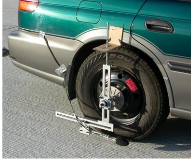
Figure 4.5 Noise Measurement Device
